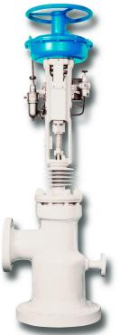
The AB6000 range of combined pressure and temperature reducing desuperheating valves provides the facility within a single unit to condition superheated steam to desired pressure and temperature levels in either steam conditioning or Turbine Bypass applications. The units can also be supplied in either in-line or angle body configuration, fixed or variable area spray unit.
